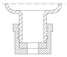
GL18-6-connector with sealing ring for 6-mm-tube
