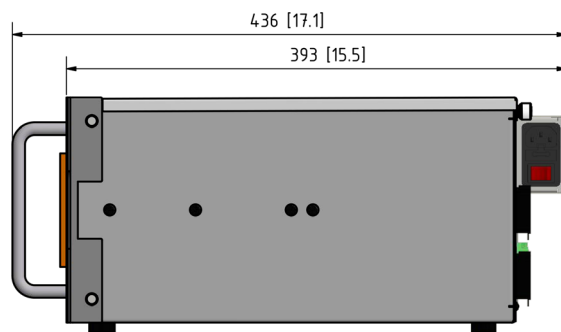
Long enclosure side view with power supply
