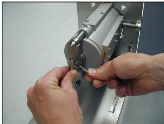
Figure 3 Dismounting the filter housing lid
