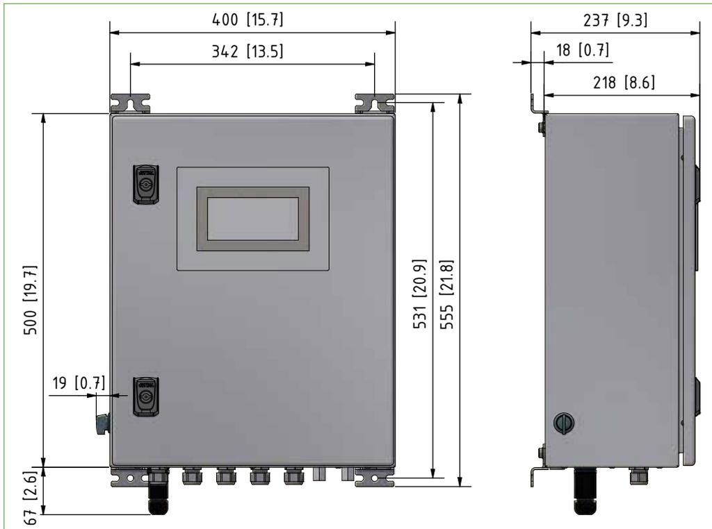
Fig. 13: Wall-mount housing, front and side-view
