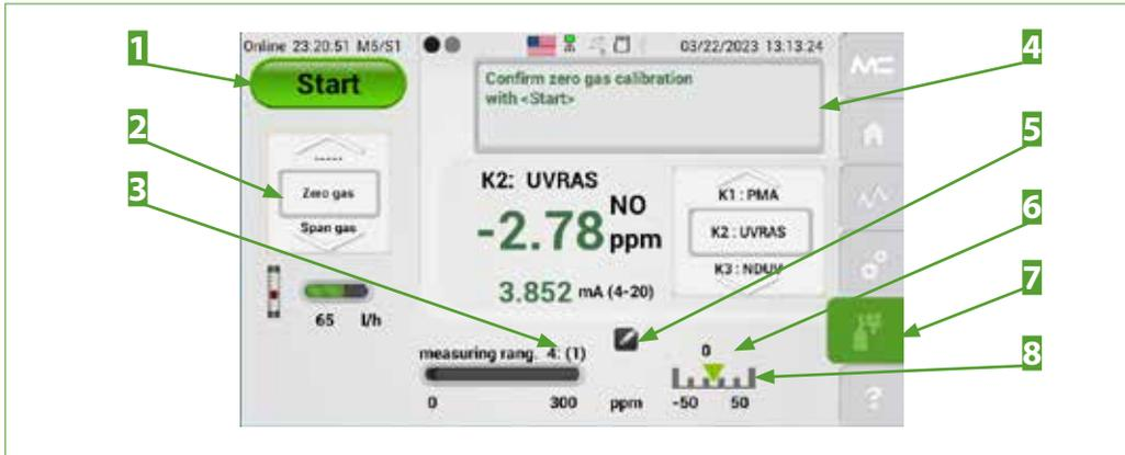
Fig. 75: Manual calibration (ManuCal)
