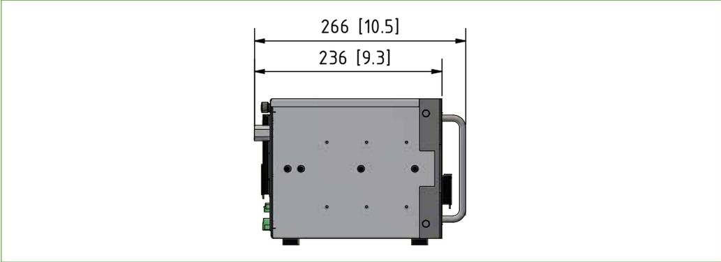
Fig. 12: 19"-rack housing side view (short housing)
