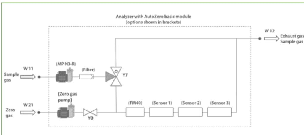
**Fig. 93: AutoZero basic module with options**
