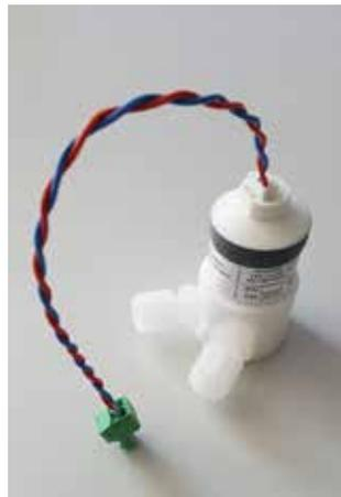
Fig. 6: Electrochemical oxygen sensor with flow chamber
