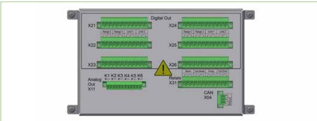
Fig. 17: Signal connections inside wall-mount device (max. equipped)
