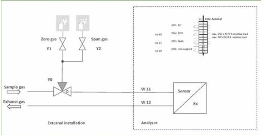
Fig. 90: AutoCal extern. valves: zero and span gas via gas cylinder
