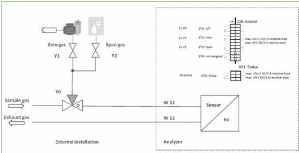
Fig. 91: AutoCal ext. valves: zero gas via filter and pump, span gas via gas cylinder
