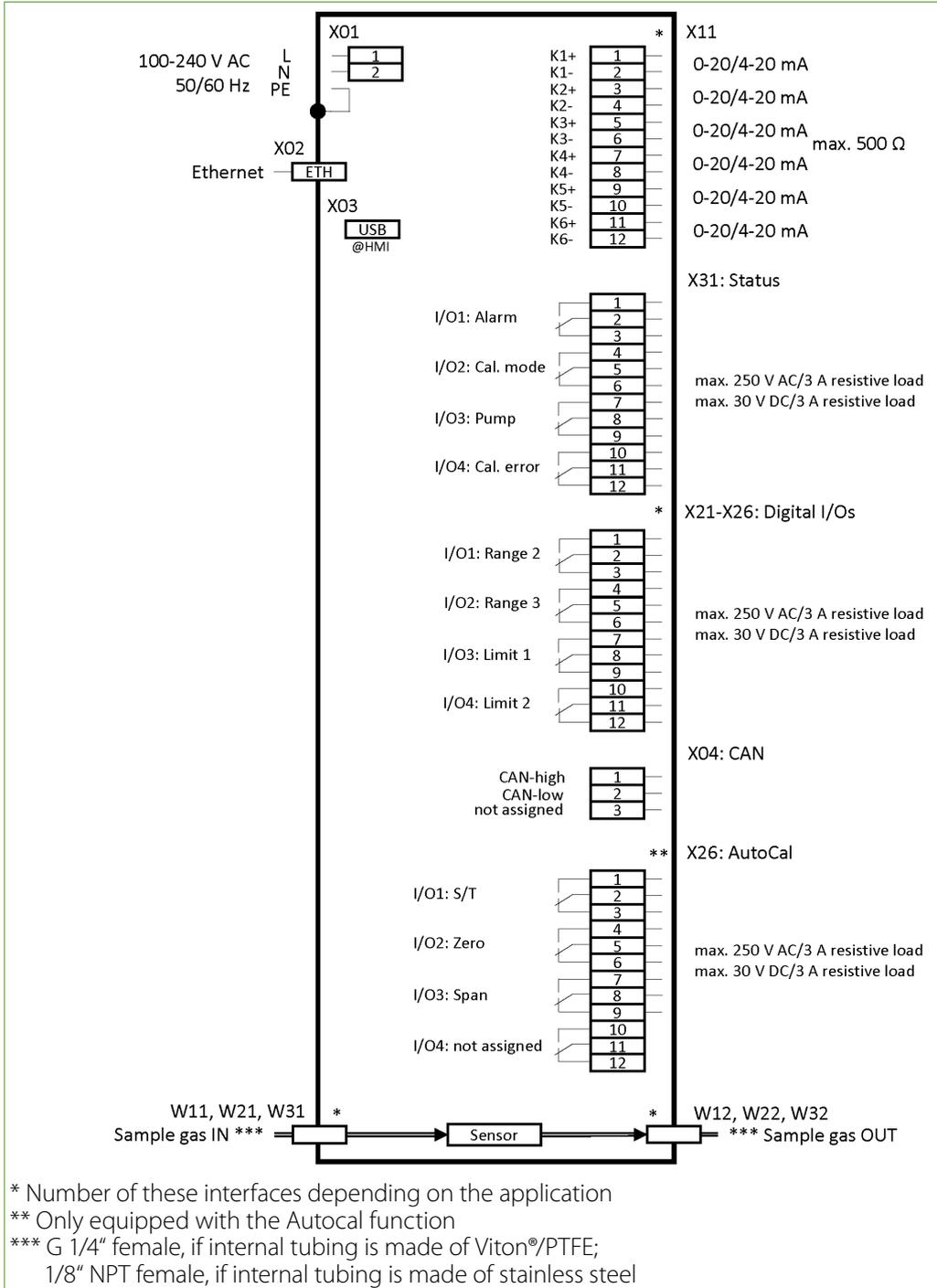
Fig. 20: Electrical interfaces: wall-mount housing
