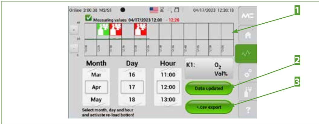
Fig. 42: M3/S1 - Recorded data selection screen
