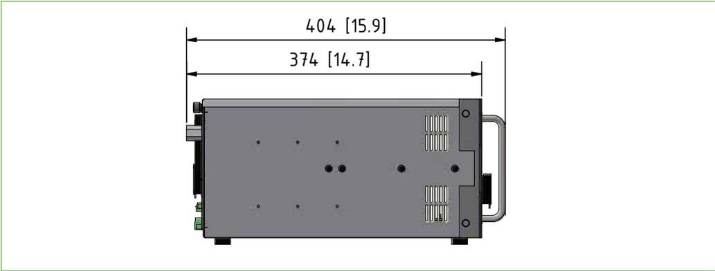
Fig. 11: 19"-rack housing side view (long housing)
