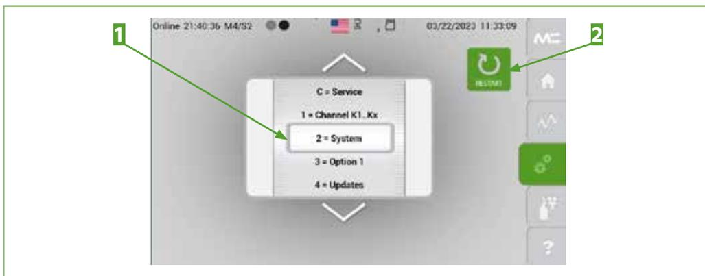
Fig. 49: M4/S2 screen with “Restart” button
