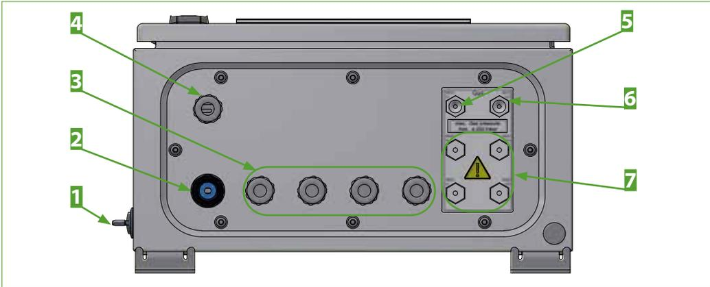
Fig. 15: Bottom-view of wall-mount device with connections
