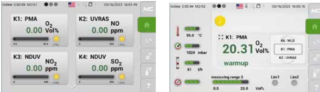
Fig. 73: Warm-up phase in M2/S1 and warm-up info on M2/S2
