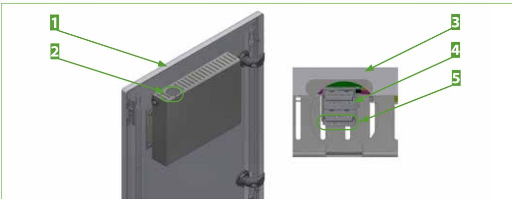
Fig. 18: Wall-mount housing: USB port for USB stick
