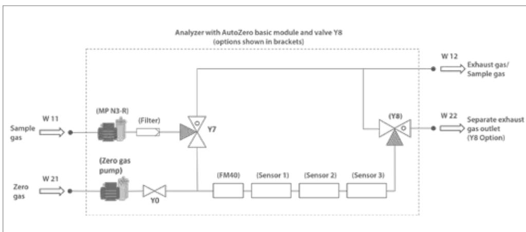
**Fig. 94: AutoZero basic module with 3/2 way valve Y8 (optionally)**
