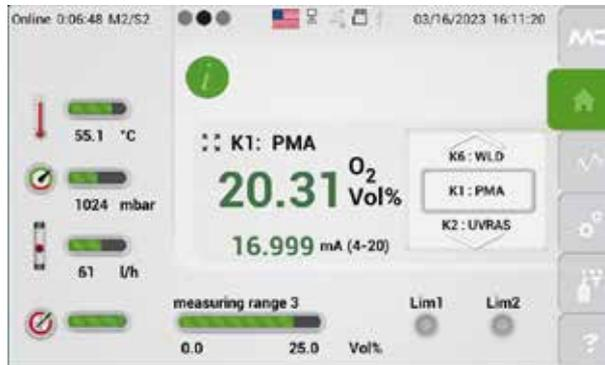
Fig. 35: M2/S2 - Detailed view of the measuring parameters
