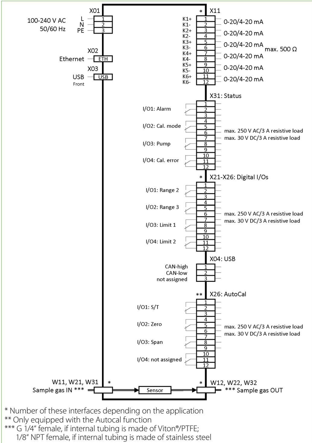
Fig. 19: Electrical interfaces: 19"-rack housing
