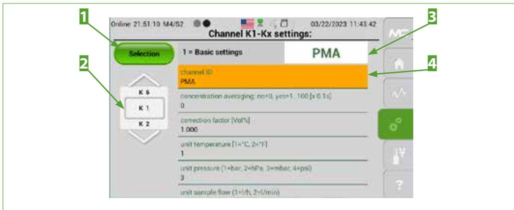
Fig. 51: Basic settings for channel 1
