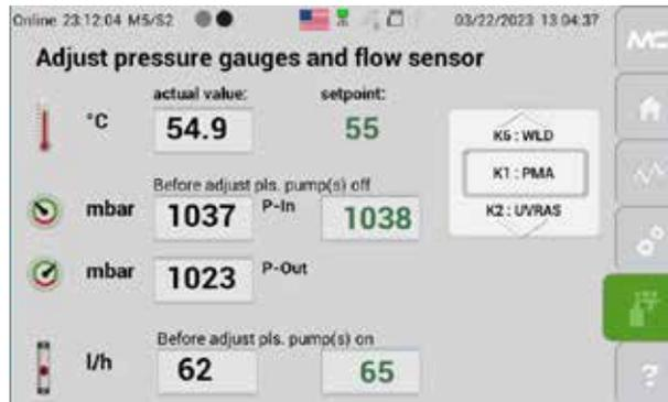
*Fig. 71: Adjust pressure gauges and flow sensor*
