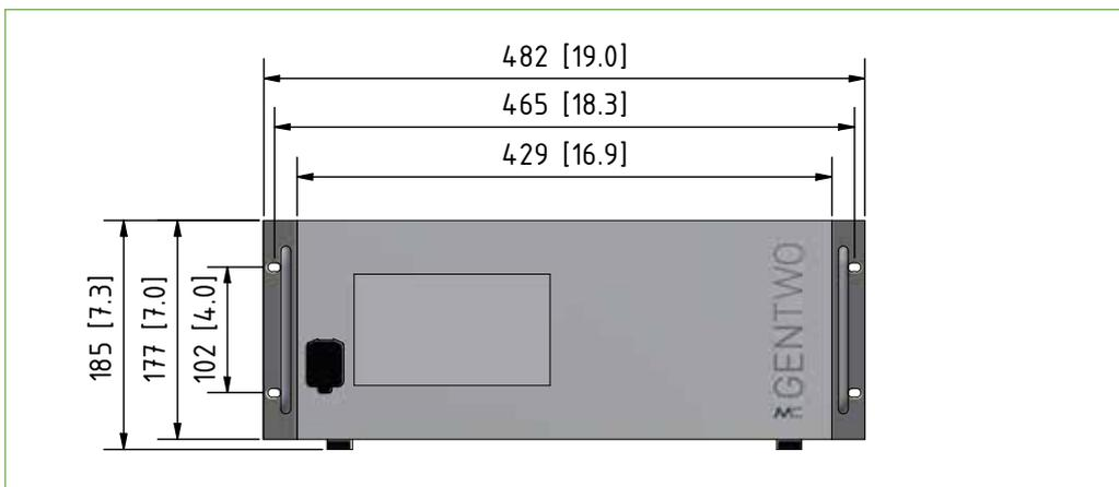
Fig. 10: 19"-rack housing front view
