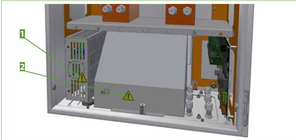
Fig. 4: Warning symbols inside wall-mount housing
