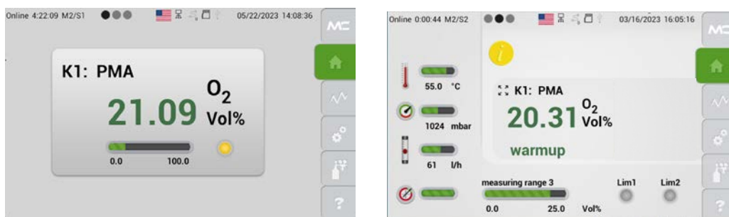
Fig. 68: Warm-up phase in M2/S1 and warm-up info on M2/S2
