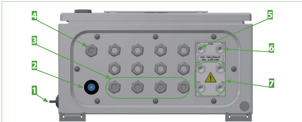
Fig. 12: Bottom-view of wall-mount device with connections
