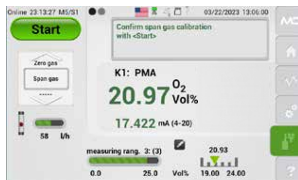
Fig. 74: Manual calibration with span gas
