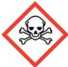
There may be harmful sample gases in the analyzer. Prevent potentially harmful gases from escaping the open probe maintenance and mounting flange. Purge this area with inert gas or air before servicing or wear appropriate personal protective equipment.
