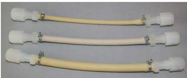
Figure 8 Different pump tube sizes (Novoprene on the left, Masterflex® on the right)
