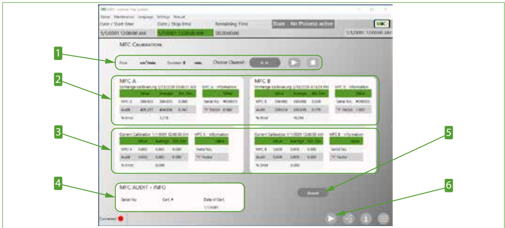
Fig. 20: Calibration of the MFCs
